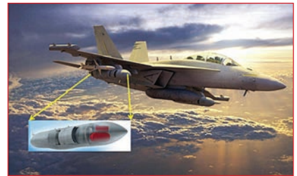
▲ Fig. 4 The Navy's Next-Generation Jammer, represents the future of EW as it uses state-of-the-art GaN devices in an electronically-steerable architecture (Source: U.S. Navy).
