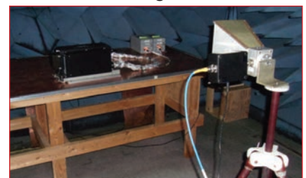
Fig. 4 Testing an RF signal recorder to MIL-STD-461.
